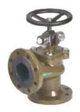
In the event of emergency or dangerous situations, quick closing valves quickly shut-off of pipe line systems carrying combustible liquids. They operate by means of remote control from outside the danger area. Under normal circumstances they are in an open position.
