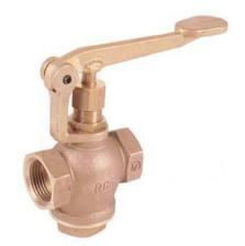
This economic self closing valve has a spring return mechanism. Used in applications where positive return to the shut-off position is required after the valve is manually opened with the pedal lever.
