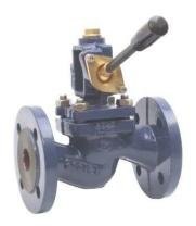
This self closing valve has a spring return mechanism. Used in applications where positive return to the shut-off position is required after the valve is manually opened with the lever.
