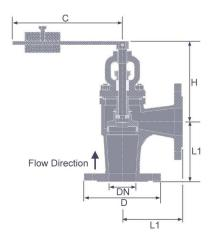
This self closing valve has a counter Features & Benefits weighted lever, they are mainly used aboard ships as a 90 degree quickly operated isolation valve.
