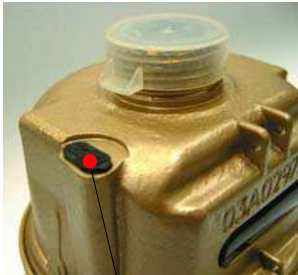
'A' Probe location position under protective plug.
