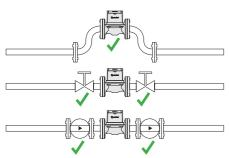
> Directly after or before 90 ° elbows, valves or pumps for meters sizes DN50-DN300 and water temperatures < 30 °C</p>
